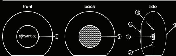
1. Power on/off 2. Micro USB charging port 3. LED indicator 4. Subwoofer 5. Speaker
